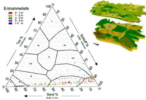
Analyzing 38 drilling cores with overall 172 soil samples
